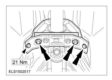
34. Align the centre bearing free of stress and tighten the bolts.
