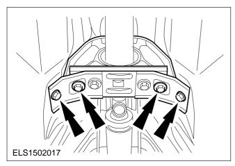
4. Release the driveshaft centre bearing.
