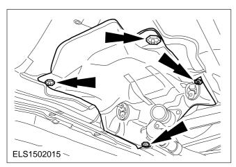
36. Fit the exhaust system front heat shield.
