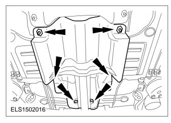
35. Fit the exhaust system rear heat shield.
