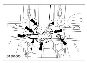
CAUTION: The driveshaft is precision-balanced by bolts of different lengths. Mark the location of the driveshafts and the bolts.
