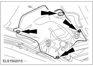
2. Detach the exhaust system front heat shield.
