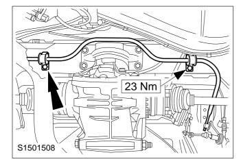
28. Fit the stabiliser (model shown up to Dec '95).
