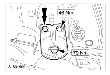
25. Tighten the bolts of the two crossmember guide plates.
