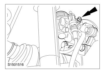
39. Bleed the brake system at both rear wheels as described in Op.no. 12 141 0.
