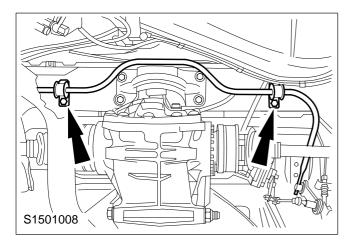
10. Detach the stabiliser bar from the bodywork (shown in vehicle up to Dec '95).
