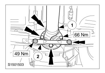
CAUTION: The driveshaft is precision-balanced by bolts of different lengths. Mark the position of the driveshaft and the bolts.
