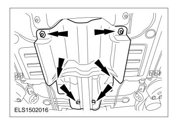
3. Detach the exhaust system rear heat shield.
