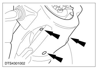
2. Remove the lower steering column shroud (three screws) (steering wheel shown removed for clarity).
