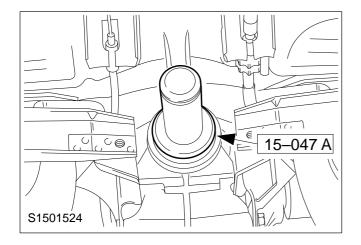
11. Fit the drive pinion flange with a new self-locking nut.
