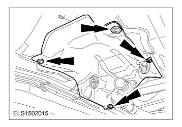
2. Detach the exhaust system front heat shield.
