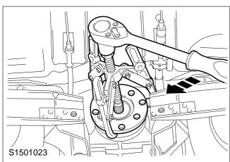
7. Pull off the drive pinion flange using a two-legged puller.
