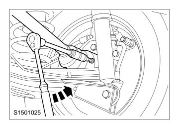
4. Detach the rear axle driveshaft from the driveshaft stub (six bolts).
