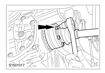
3. Detach the rear axle driveshaft from the differential (vehicle shown built up to Jan '95).
